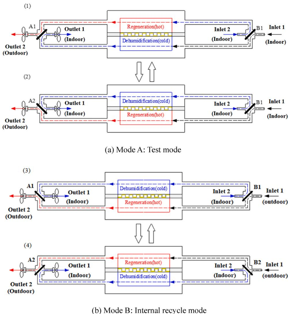
Fig. 4. The operation modes of MOF humidity pump.
