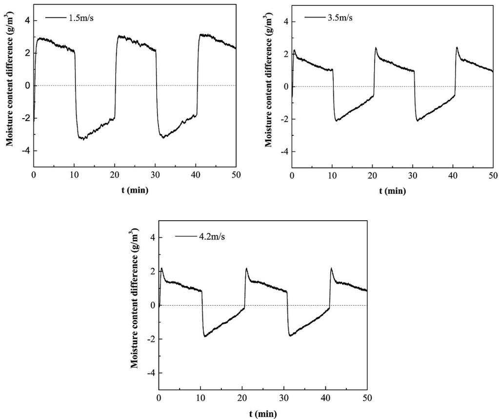
Fig. 11. Moisture content difference of humidity pump with different air velocity.
