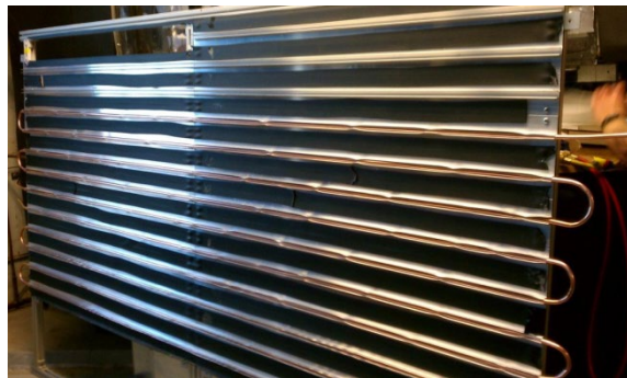
Copper tubes at the back of RHX
