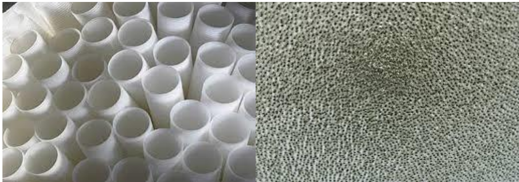
Figure 7.13 porous material idealized as a collection of cylindrical tubes.
